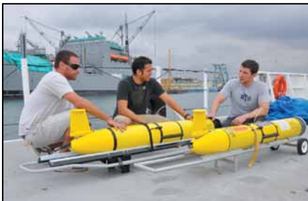
Engineers prepare Naval Oceanographic Office sea gliders for collecting underwater data that will be used in developing ocean forecasts.
